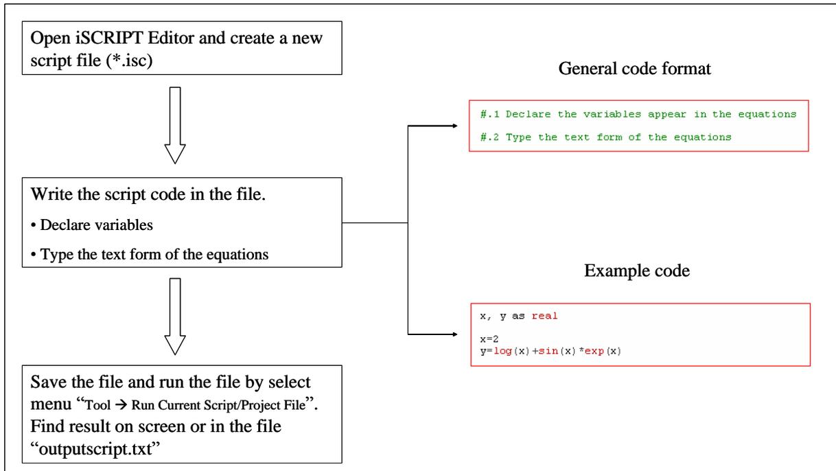
Figure 3.1. The basic procedure for solving an arithmetic and algebraic problem in iSCRIPT.
