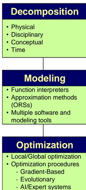
**Figure 1.1.** Tasks in a multi-level design/optimization analysis.
