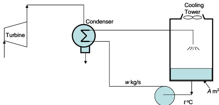
Figure 5.8. Cooling tower, pump, and condenser system of a heat rejection system.
