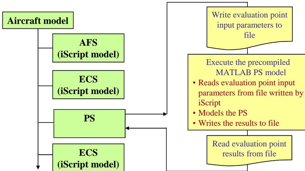
Figure 7.2. An aircraft model with the PS subsystem modeled in a software or executable outside of iSCRIPT.
