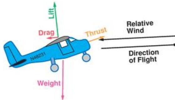
Figure 4.4 Aerodynamics Forces on an Aircraft
