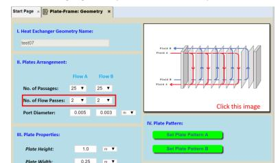
When defining the heat exchanger geometry, the number of flow passes can be defined:
