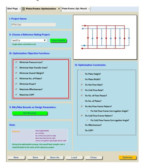
Similar to the Sizing module, after specifying the bounds on the design parameters and chosing the design constraints, you can click the "Compute" button to start the Optimization calculations. When the calculations have been completed, all possible design realizations that satisfy the design target will be listed in a table. The list of the realizations is sorted based on how well the realizations satisfy the optimization targets. The best one is placed at the top of the table.
