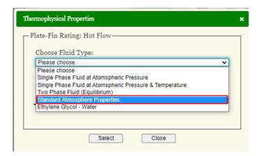
The "Standard Atmosphere Properties" data will be displayed. The properties of atmospheric air at the specified altitude will be calculated after you have specified a value for the altitude.
