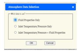
If you select the "Fluid Properties Only" option, after clicking the "OK" button, only the fluid thermophysical properties (dynamic viscosity, specific heat at constant pressure, thermal conductivity, and density) will be loaded into your project.
