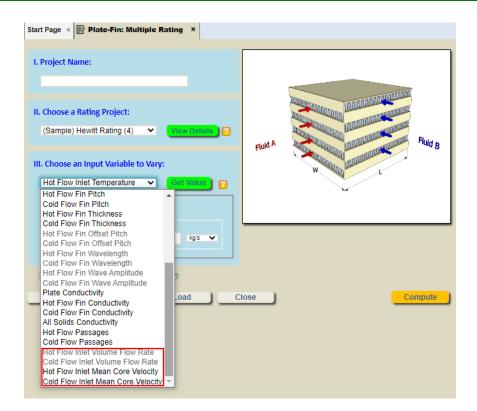
Note that only the flow rate type chosen in the reference rating project can be activated in Multiple Rating, and the options for other types of flow rate specification will be greyed out.
