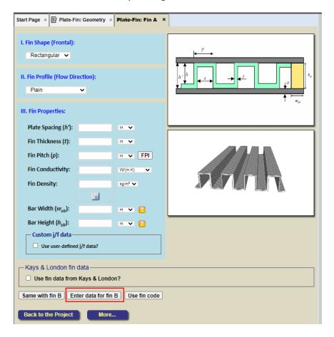
• Similarly, the "Enter data for fin A" button has also been added to the tab for Fin-B, which directly takes you to the tab for Fin-A.
