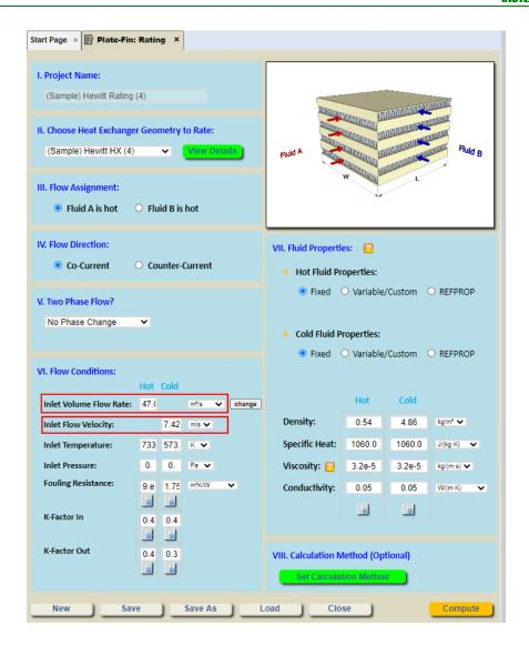
3) The "Hot/Cold Flow Volume Flow Rate" and "Hot/Cold Core Mean Velocity" options have also been added to the **Multiple Rating** task to allow the range of flow rate to be used in the chosen input type during the calculation.
