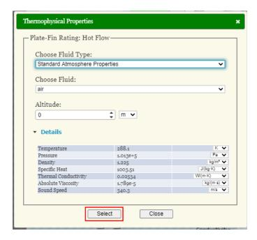
The data for the **fixed fluid properties** can be obtained directly for atmospheric air in the database by clicking on the "**Select**" button. When you do this, you are presented with three options:
