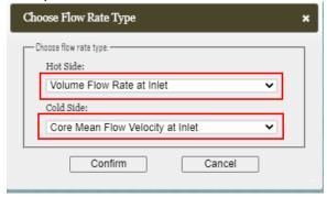
After selecting the flow rate type for each stream, the corresponding input textboxes will be displayed to allow you to enter the values of the chosen type of flow rate.
