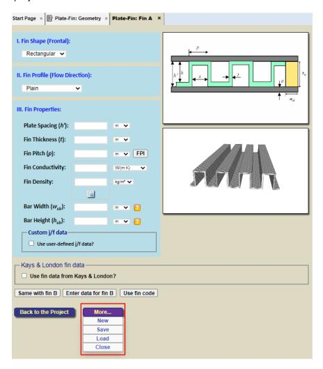
• Note that the menu buttons "New/Save/Load/Close" have the same functions as those in the main heat exchanger geometry tab.
