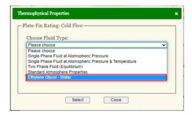
The **Ethylene Glycol/Water** data will be displayed. The ethylene glycol/water mixture properties will be calculated when you specify the values of the temperature and percentage weight (or volume) of ethylene glycol.
