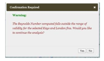
If "No" is selected in the dialog box (above), the run will be terminated. If "Yes" is selected, the calculation will continue, and an extrapolation will be used to calculate the j/f data beyond the data points of the Kays and London fins. Obviously, the you must pay particular attention to the analysis results you obtain by "forcing" a solution beyond the database.
