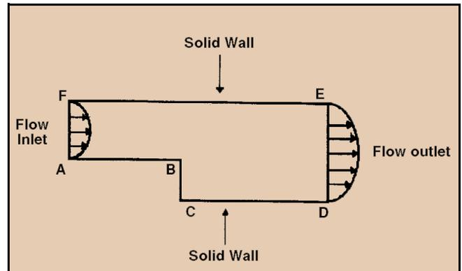
Figure 1: The physical model for the flow of air in a backward-facing duct.
