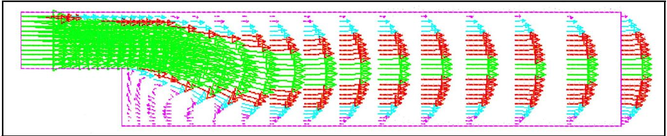
**Figure 3: Velocity vectors for the flow of air in a duct. Calculations were done with a commercial CFD code.**
