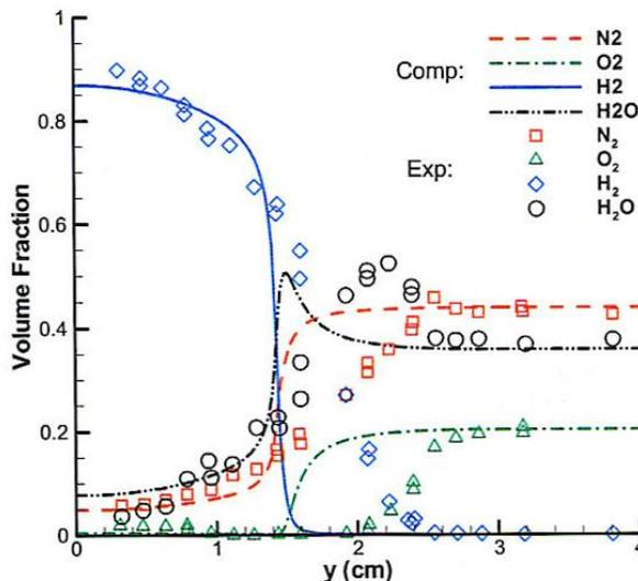
**Figure 4. Composition profiles, reacting case, variable  $Sc_t$ , ( $Pr_t = 0.5$ ),  $k-\zeta$  model, with turbulence/chemistry interaction (Ref [71]).**
