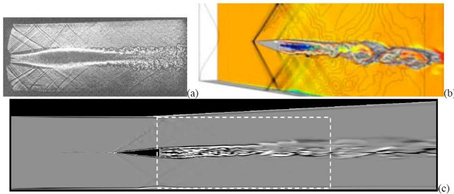
Figure 6. Results from Berglund et al.<sup>92</sup> for supersonic flow in the scramjet combustor with hydrogen injection and combustion. a) Shadowgraph photographs from the experiments, b) a perspective view from the rear of the simulated flow and c) a numerical shadowgraph image from the reacting LES calculations. The size and location of the experimental image a) is superimposed on c).
