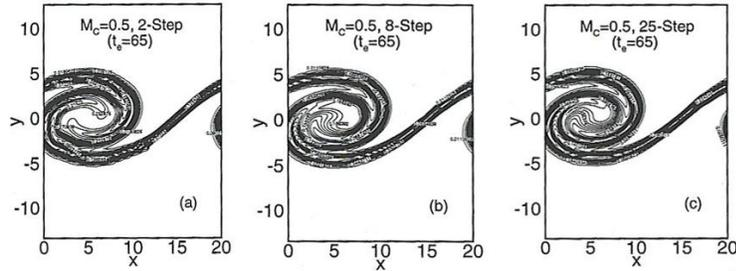
**Figure 3. Contour maps of water mass fraction for supersonic combustion in mixing layers as a function of the kinetic model. Results were obtained from a transported joint PDF for supersonic combustion (Ref [45]). The various kinetic mechanisms are given in the appendix.**
