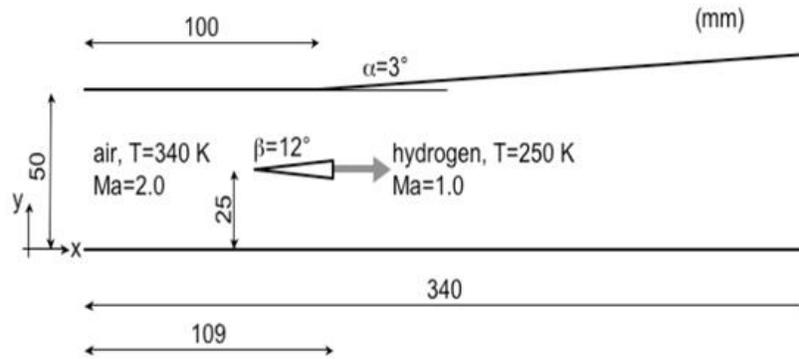
Figure 5. Schematic of the computational domain of the DLR scramjet model in Berglund and Fureby.<sup>92</sup>
