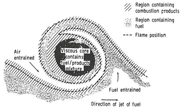
**Figure 1. Cross section of transitional “vortex” eddy in gas diffusion flame (Ref [32]).**
