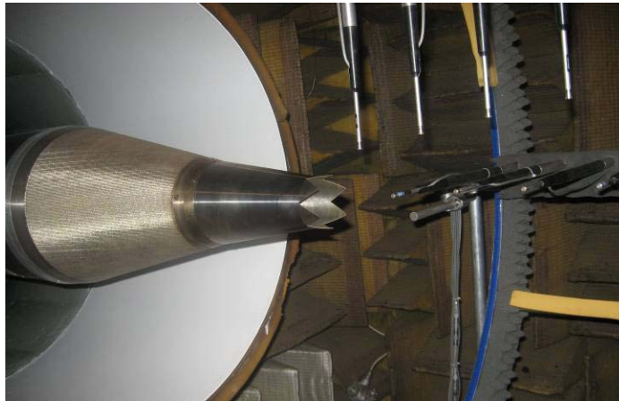
Figure 4. Converging-diverging chevron nozzle with fixed and rotating near field microphones in field of view.
