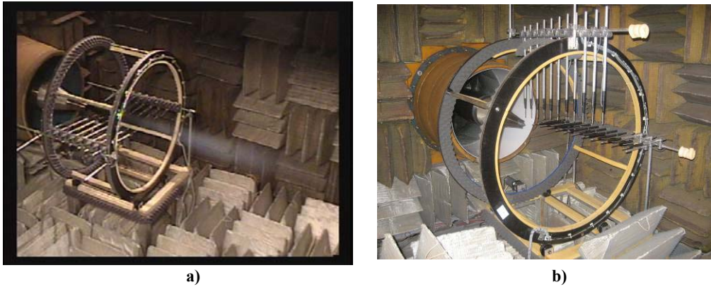
Figure 1. a) Rotating array configuration installed in UTRC Acoustic Research Tunnel b) view looking upstream into 36 inch diameter open jet wind tunnel with rotating array in vertical plane perpendicular to reference microphones
