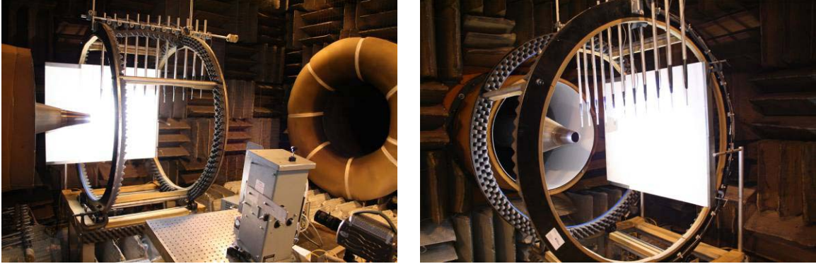
Figure 7. Shadowgraph system installed in ART with large retro-reflective image plane and near field microphone rotating array.
